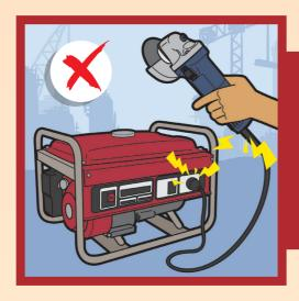
It is dangerous to use a portable generator for any hand-held tool with a metallic casing
