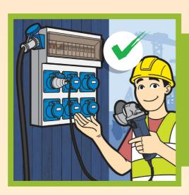
A Socket-outlet Assembly (SOA) provides industrial socket-outlets for easy and safe tapping of electricity supply. The built-in electrical protective devices further enhance safety in the use of hand-held tools and electrical equipment
